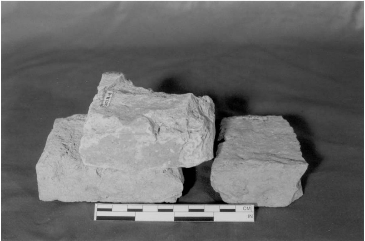
Plate 23. Small brick type of Dutch origin referred to as drielingen recovered from Feature 20.
