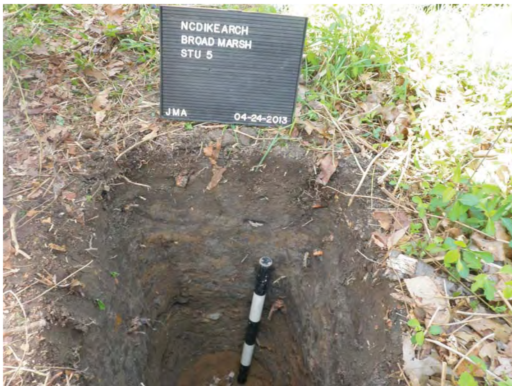
Plate 2. STU 5 at the Broad Marsh Dike, showing the mix of upland and marsh soils used to construct the dike.
